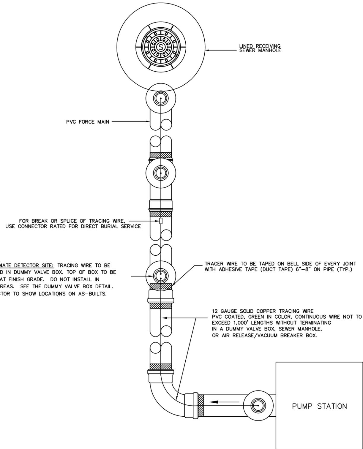
***TRACING WIRE INSTALLATION DETAIL***
